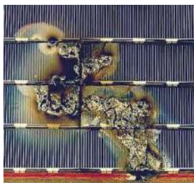
FIGURE 3. The damage of solar array caused by arcing in ESA EURECA [14].
