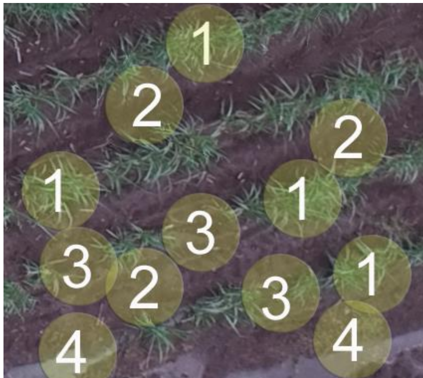
Figure 2: Identification of missing vegetation from a crop field. Areas labeled as (1) represent examples of sugar cane plants while areas labeled as (2) constitute examples of soil. Areas (3) depict missing vegetation examples, i.e. it should have been sugar cane but it is soil. Finally, areas (4) are examples of “Others”, being irrelevant image segments.
