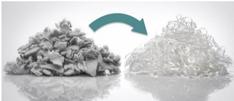
Figure 5. Glass fibre waste material before and after recycling [92]
