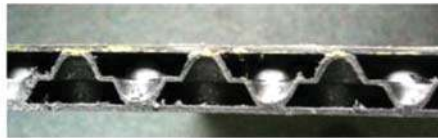
Fig. 14. Polypropylene thermal absorber with honeycomb structure for PV/T module [31].
