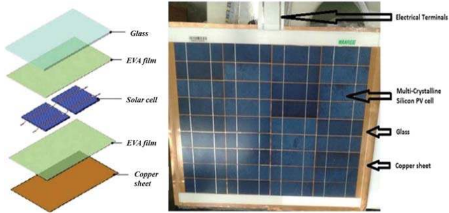
Fig. 29. Combine PV layer with thermal absorber by EVA lamination without TPT back sheet [97].
