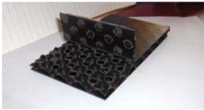
Fig. 14. Polypropylene thermal absorber with honeycomb structure for PV/T module [31].
