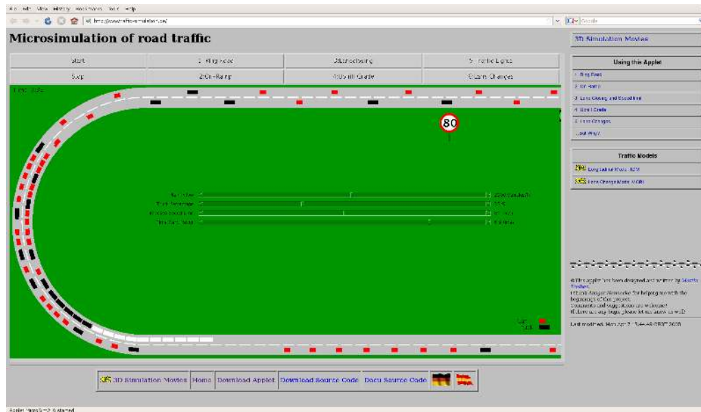
Figure 5: Treiber's Microsimulation of Road Traffic - illustrating the use of different types of vehicles used in the simulation: cars and trucks. The cars are represented with smaller rectangles in red color, while the trucks are larger rectangles in black color [14]
