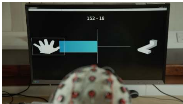
Figure 2. Example of feedback often provided to users during MT-BCI training. In this example, the user has to train to imagine left-hand movement, performing mental calculation and imagining an object rotating [171]. At the moment the picture was taken, the user had to imagine moving their left-hand. The blue bar location and direction indicates the task which has been recognized. The bar length indicates how confident the system is in its recognition: the longer the bar, the more confident the system. Here the system correctly recognizes the task that the user is performing and is quite confident about it.
