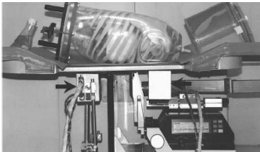
Fig. 19 PEM detectors installed on an autopsy system [42]
