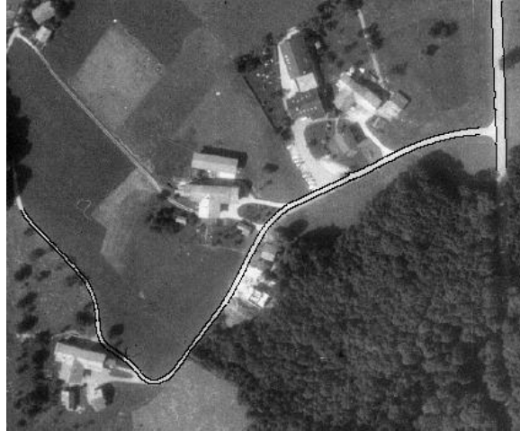
Figure 19: Extracted roads from an aerial image (Reproduced from [Mayer et al. 1997])
