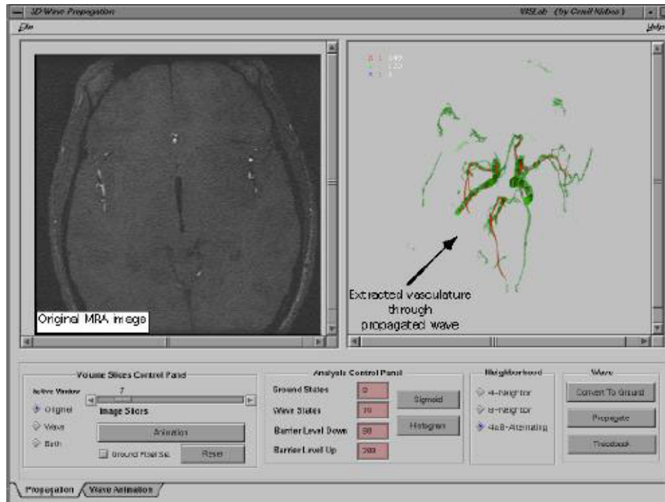
Figure 10: Extracted vessel tree using 3D wave propagation
