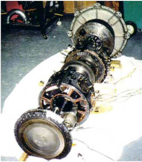
Fig. 14 Disassembled view of the GPC rotor, taken from Ref. [137]
