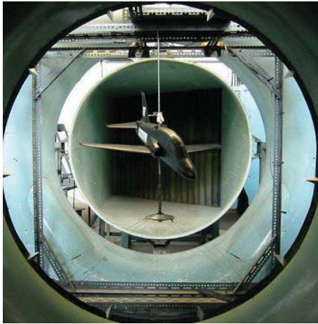
FIGURE 17: Four-degree-of-freedom support rig in a low speed open-section wind tunnel [101].
