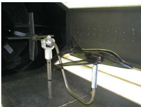
FIGURE 19: The 5-DOF rig mounted in the University of Bristol's 7 × 5 ft closed-section wind tunnel [108].
