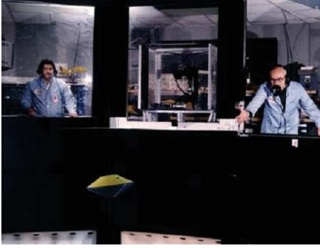
FIGURE 7: Return capsule model performing free fall motions in a VST [7].
