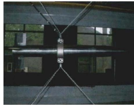
FIGURE 26: The first VFT system built by CAAA in China [118].
