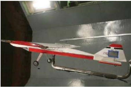
FIGURE 4: An UAV aircraft mounted on a forced oscillation rig [12].
