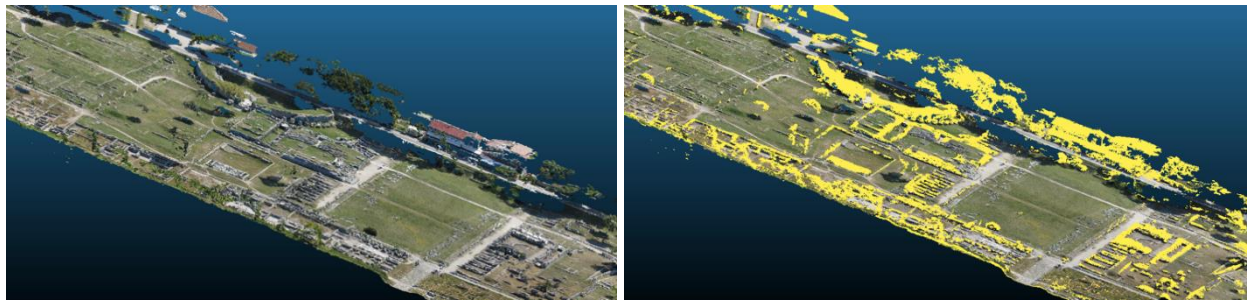
Figure 5: 3D point cloud of the archaeological site of Paestum (left) and segmentation to separate bare earth and man-made structures (right).
