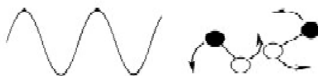
Fig:-1. Dipolar molecules which try to align with an oscillating electric field
