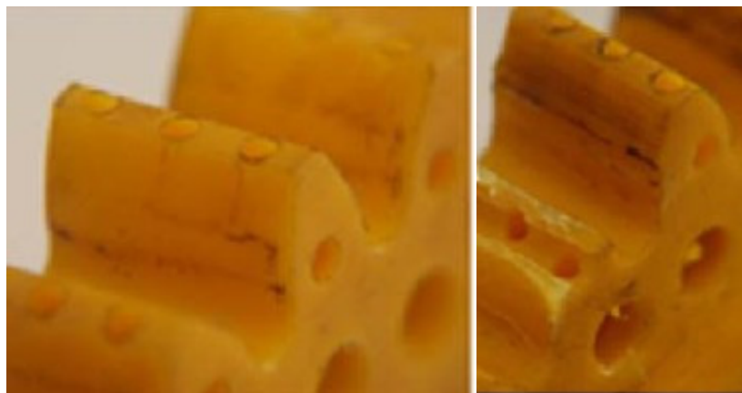
Figure 2. The damage in newly designed gears (Hayrettin, 2009)
