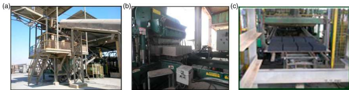
FIGURE 16. (a) Photograph of a precasting plant; Production of (b) type 14 wall blocks (c) type 6 pavers.
