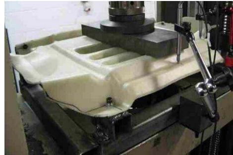
Fig. 4: Flax/PLA interior floor-well panel Fig. 5: Frame for holding the foot-well panel
