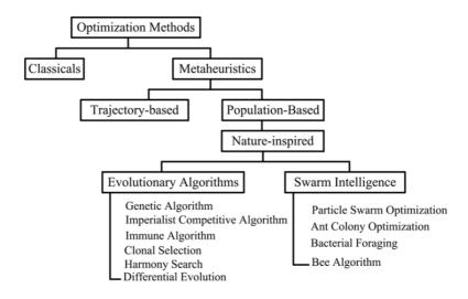
Figure 2. Metaheuristics Optimization Methods Classification [29]
