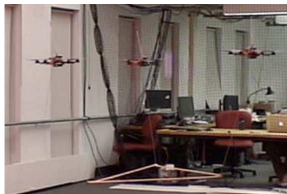
Figure 11 Under-constrained CDPR of multiple aerial robots
