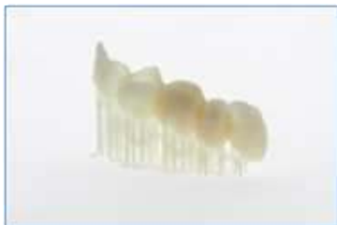
Figure 3. Additively manufactured interim dental restoration before the removal of the supportive structures.
