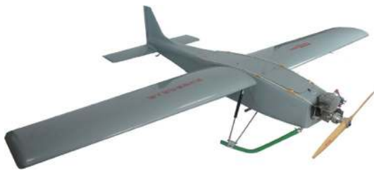
Fig. 1 The KC2800 is a fixed-wing drone used for surveillance and mapping. Picture reprinted from https://aibirduav.diytrade.com
