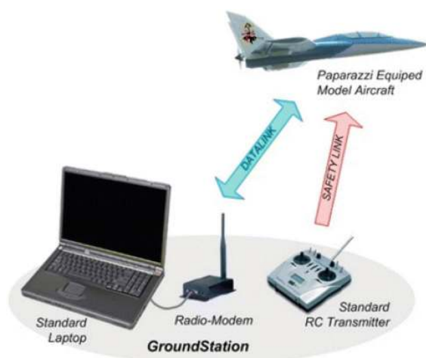
Fig. 10 Platform for drone control from GCS . Picture reprinted from https://www.google.com/search?q=multirotor+UAV++ground+control+station+images
