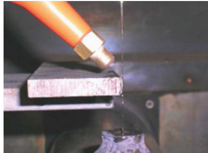
FIGURE 14. Near dry wire EDM with air-water mixture [23].
