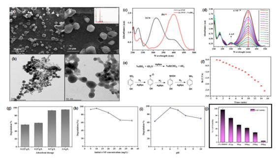
**Figure 7.** (**a**) SEM analysis. The EDX insert shows that the formed nanoparticles are silver. (**b**) TEM image showing the synthesized AgNPs using B. amyloliquefaciens. (**c**) Absorption spectra of 4-nitrophenol in aqueous medium and 4-nitrophenol+NaBH<sub>4</sub> in aqueous solution. (**d**) Absorption
