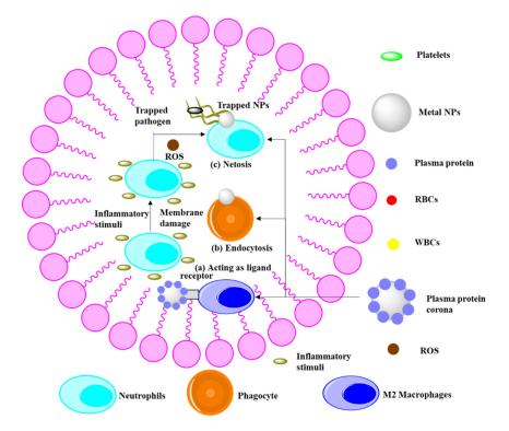
Figure 3. Anti-inflammatory mechanism adopted by various nanoparticles.
