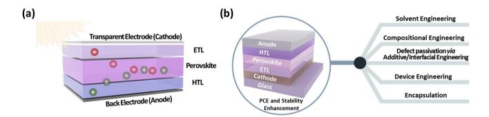
Fig. 2 Schematics showing a stacking of different layers in a typical PSC and b the prominent ways for improving PCE and stability of PSCs
