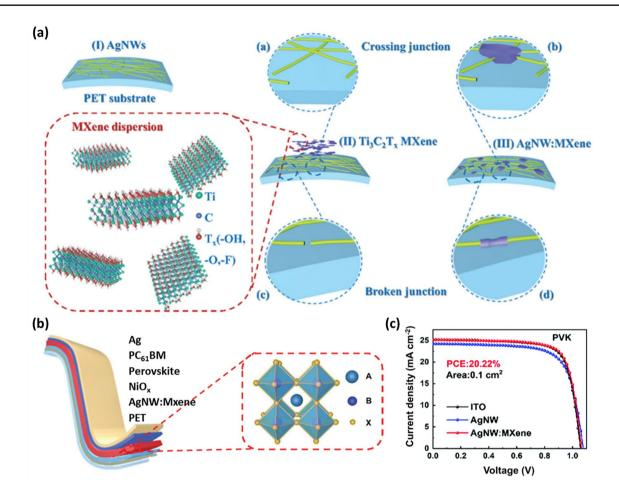
**Fig. 12** a Schematic of the  $Ti_3C_2T_x$  MXene and the fabrication procedure of AgNW:MXene flexible transparent conductive electrodes. **b** Flexible PSCs with the structure of PET/AgNW:MXene/NiO<sub>x</sub>/Perovskite/PC<sub>61</sub>BM/Ag. **c** *J*–*V* curves of the flexible PSCs based on ITO, AgNW, and AgNW:MXene electrodes [176]. Copyright © 2022 The Royal Society of Chemistry
