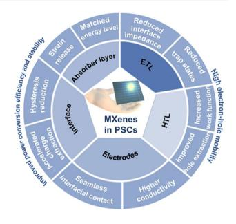
Fig. 17 Positions and functions of MXenes in PSCs
