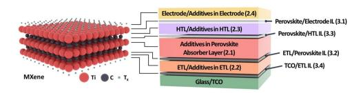
Fig. 3 MXenes in PSCs: Various roles of MXenes as components or parts of the components in regular n-i-p PSCs. The device structure of Glass/TCO/ETL/Perovskite/HTL/Electrode with different ILs, positions of MXenes and numbers in the parenthesis indicate the Section numbers. IL stands for "interfacial layer," and TCO stands for "transparent conducting oxide"
