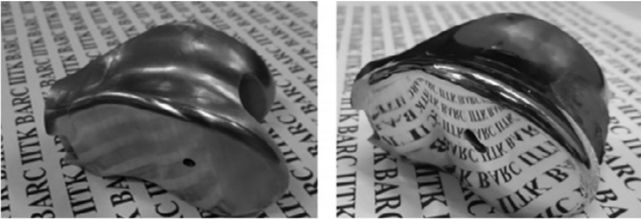
Fig. 17. Knee joint implant before and after finishing [80].
