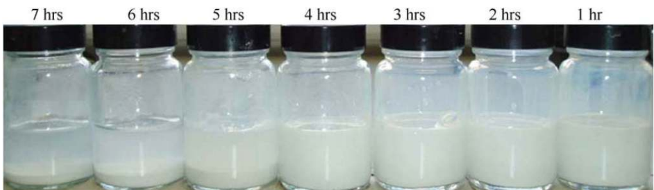
Fig. 2 Sedimentation of \text{Al}_2\text{O}_3 nanoparticles without stabilizer [23]
