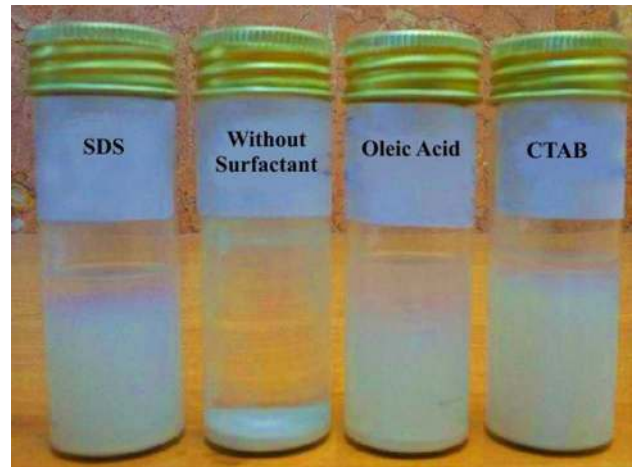
Fig. 4 Effect of surfactant on Mg(OH) 2 / water nanofluid (after 30 days) [46]
