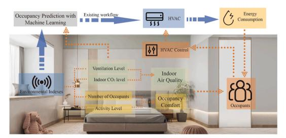
Fig. 8. The existing workflow of IAQ and thermal comfort prediction and the potential improvement.
