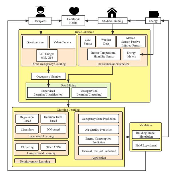
Fig. 3. The typical procedure of occupancy prediction with machine learning, validation and applications in the built environment.
