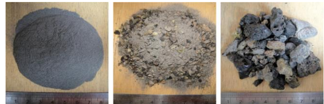
Fig. 1 Typical particle sizes of coal bottom ash [1]
