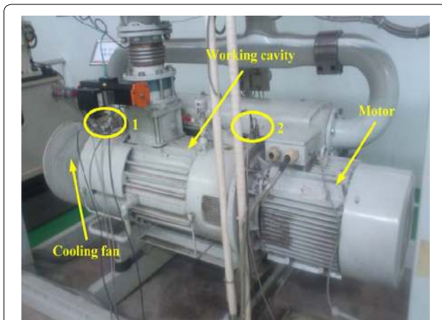
Figure 9 Vacuum pump test-bed
