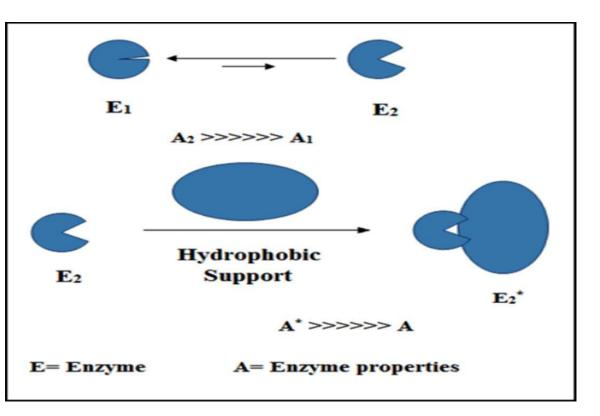
**Figure 2:** Cleavage of dimers and immobilization on hydrophobic supports (in the absence of hydrophobic surfaces, molecules of lipase forms dimers, however a hydrophobic surface can split them again).
