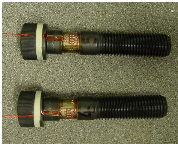
Figure 2: A sample bolt with electrical strain gauge.
