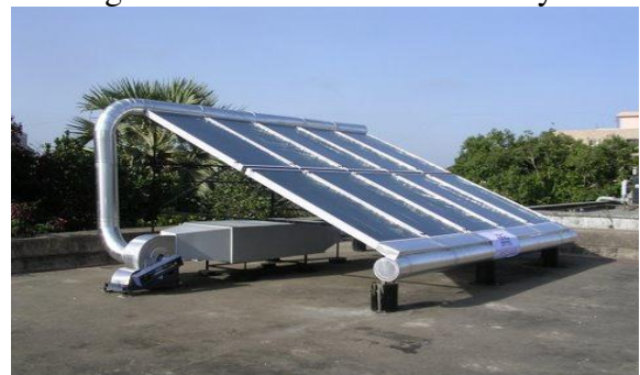
“Figure 3. Schematic view of indirect type solar dryer”
