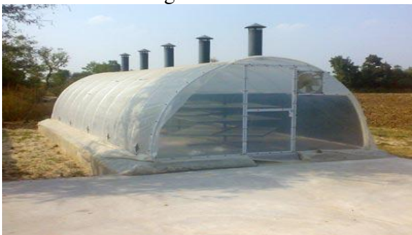
“Figure 2. Schematic view of direct type solar dryer”
