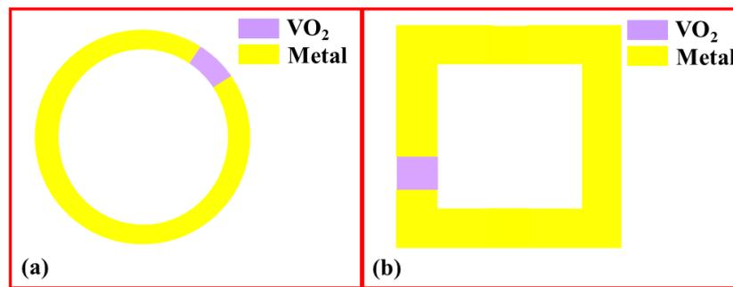
**Figure 11.** Metamaterial polarization converters based on (a) circular split ring resonator structure; (b) square split ring resonator structure.
