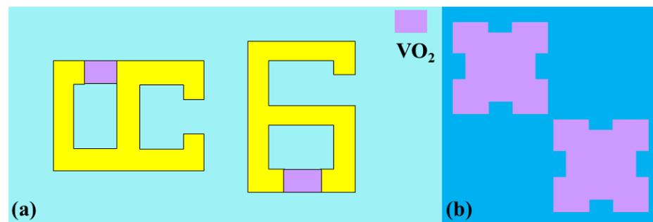
**Figure 10.** VO<sub>2</sub>-based metamaterial absorber structures. (a) Split-ring metal resonators with embedded VO<sub>2</sub> material [138]; (b) two VO<sub>2</sub> patterns [147].
