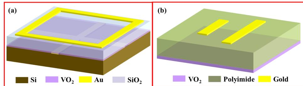
**Figure 15.** VO<sub>2</sub>-based transmissive metamaterial structures. (a) Structure designed by L. L. Chen et al. [157]; (b) structure designed by C. X. Liu et al. [159].
