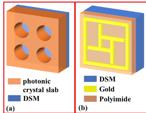
**Figure 16.** DSM-based metamaterial absorbers. (a) Photonic slabs with a thick DSM film [172]; (b) bulk DSM film layer [173].
