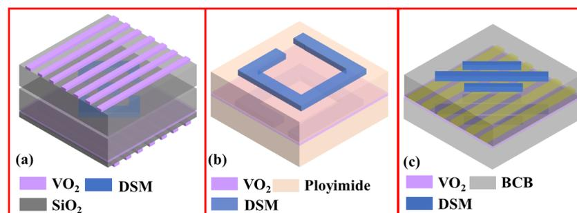
**Figure 18.** Multi-functional metamaterial structures based on the combination of VO<sub>2</sub> and DSM. (a) LTL and LTC polarization converter [176]; (b) asymmetric transmission and dual-directional absorption [177]; (c) polarization conversion and reflection device [178].
