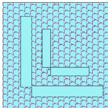
**Figure 8.** Graphene-based terahertz metamaterial polarization converter composed of graphene monolayer etched with pairs of rectangles [96].
