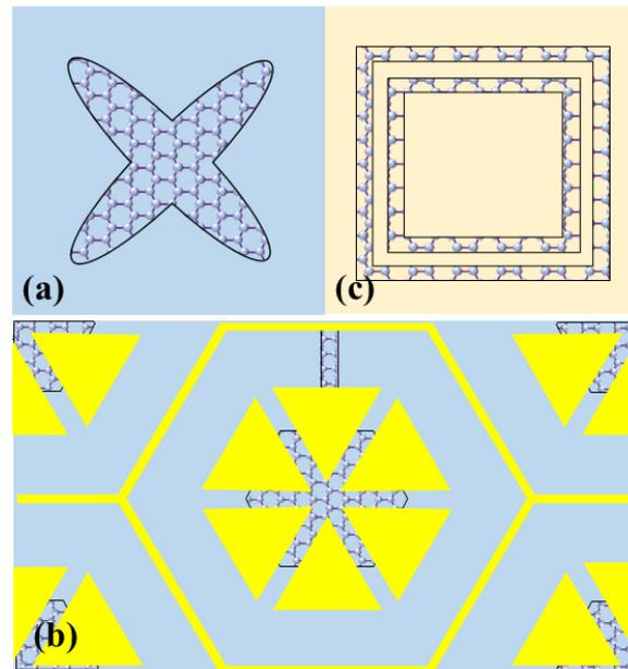
**Figure 3.** Graphene-based multi-band terahertz metamaterial absorbers using discrete graphene microstructures. (a) cross-elliptical graphene pattern [37]; (b) hybrid graphene-gold structure [50]; (c) double graphene square ring. Adapted with permission from Ref. [51], 2019, Copyright The author.
