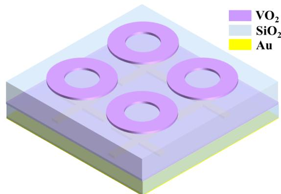
**Figure 12.** VO<sub>2</sub>-based broad-band absorption and narrow-band absorption structure [151].
