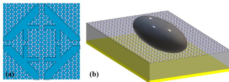
**Figure 6.** Graphene-based broad-band terahertz metamaterial absorbers. (a) structure designed by J. Z. Han et al. [78]; (b) a Si semi-ellipsoidal structure on a single-layer graphene film [83].
