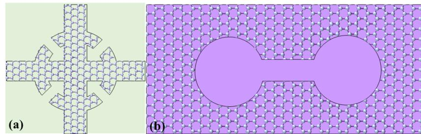
**Figure 4.** Graphene-based multi-band terahertz metamaterial absorbers using continuous graphene microstructures. (a) Graphene crossing and graphene ring with four gaps [54]; (b) dumbbell-shaped structure graphene [55].
