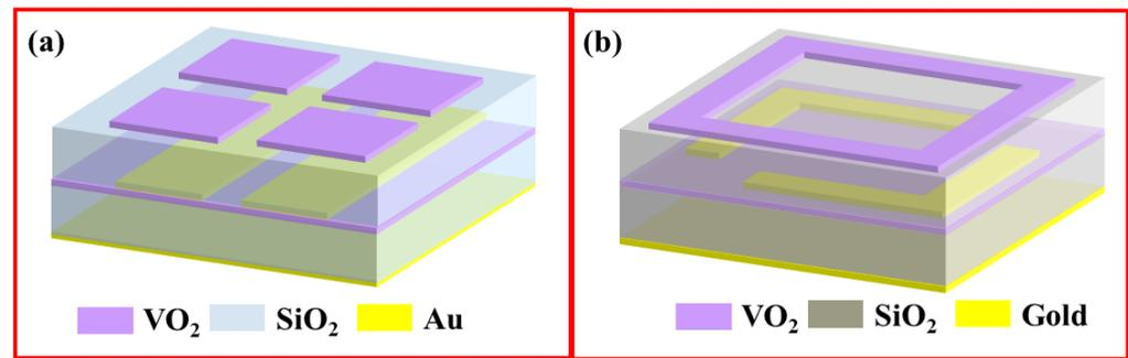
**Figure 13.** VO<sub>2</sub>-based metamaterial structures realizing absorption and polarization. (a) Proposed by Z. Y. Song et al. [152]. (b) Proposed by our group [153].
