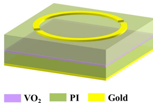
**Figure 14.** Nonstructured VO<sub>2</sub> film-based metamaterial multi-functional polarization structure. Adapted with permission from Ref. [156], 2022, Copyright the author.
