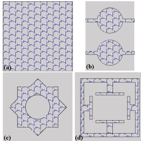
**Figure 2.** Graphene-based single-frequency/band terahertz metamaterial absorbers. (a) Metal wire and continuous graphene film; (b) two identical-sized graphene disc elements [31]; (c) square-square-circle graphene microstructure [32]; (d) four T-shaped graphene strips and a graphene square ring. Adapted with permission from Ref. [33], 2019, Copyright The author.
