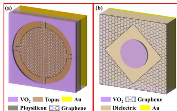
**Figure 19.** Multi-functional metamaterial structures based on the combination of VO<sub>2</sub> and graphene. (a) Realizing absorption with different characteristics [179]; (b) realizing absorption and polarization conversion [189].
