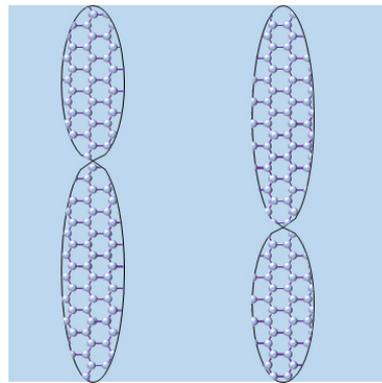
**Figure 7.** Broad-band terahertz metamaterial absorber based on asymmetric oval-shaped graphene patterns [91].
