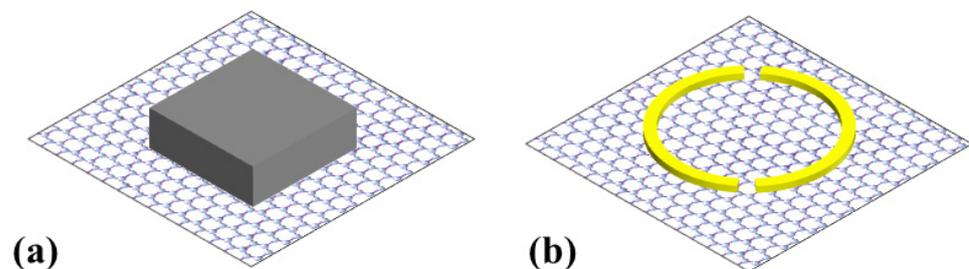
**Figure 5.** Graphene-based multi-band terahertz metamaterial absorbers using nonstructured graphene film. (a) dielectric-graphene-based structure; (b) Hybrid metal-graphene-based structure.
