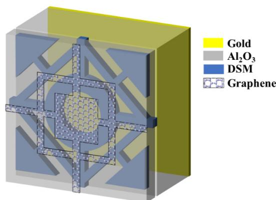
**Figure 20.** Designed absorber based on the combination of DSM and graphene [169].
