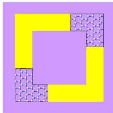
**Figure 9.** Metamaterial polarization converter structures based on double-split graphene ring [111].
