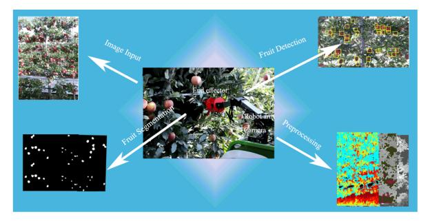
Figure 4. General architecture of IoT-based fruit detection for harvesting.
