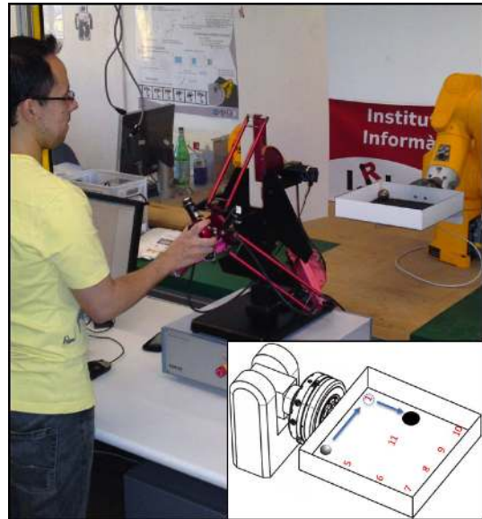
Fig. 2 Experimental scenario of the ball-in-box task. (At the bottom right corner) Initial positions of the ball for the training phase and motion strategy followed by the teacher. Numbering is counterclockwise.
