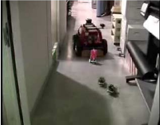
Fig. 3: The Parent robot deploys the smaller robots through a doorway into a large DOE facility.
