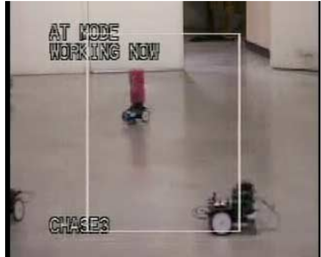
Fig. 4: The view from the Parent robot. The operator uses this feedback to guide the sergeant through the door as the privates swarm behind it.
