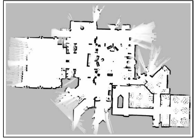
Figure 2: A map of the testing facility, the Longwood Retirement Resort in Oakmont, PA. This map has been acquired by our mobile robot. It exhibits a range of different areas, such as a dining hall (right) and a conference hall (left).
