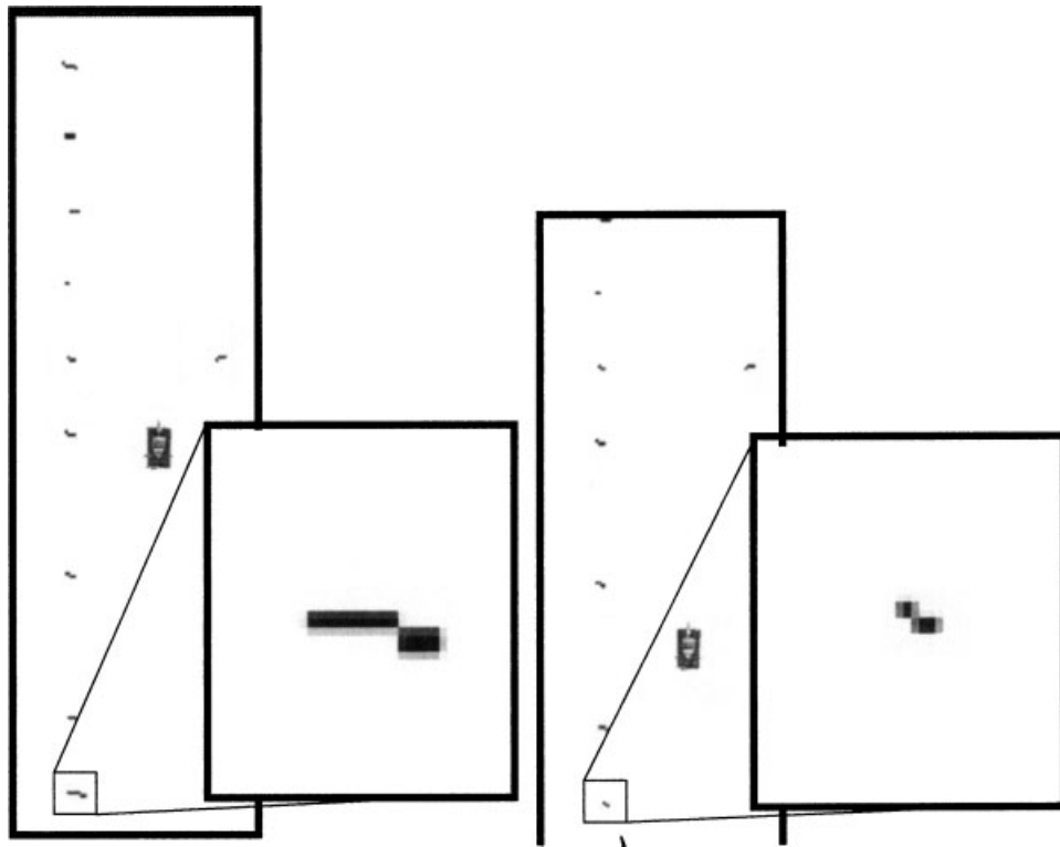
Figure 21. Two maps recorded driving along a barbed-wire fence during the 2005 Grand Challenge. The left map shows the magnified fence post at 35 m range. The right map shows the same post, this time at 15 m range. As the obstacle approaches, its size and position are refined, while obstacles behind the vehicle and out of the antenna's field of view are retained.
