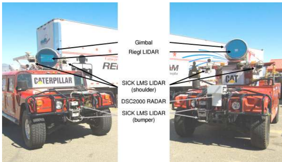
Figure 12. H1ghlander (left) and Sandstorm with their sensors labeled.
