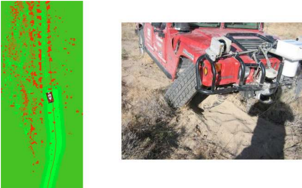
Figure 22. An example of incomplete data (a) which led to significant damage (b). The red continuous line represents the preplanned path. The data show that the preplanned path is on the road edge and veers off the road, which is combined with the with the hill crest to cause the robot to leave the road.
