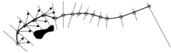
Figure 25. The conformal planner operates between cells on adjacent segments normal to the preplanned path.
