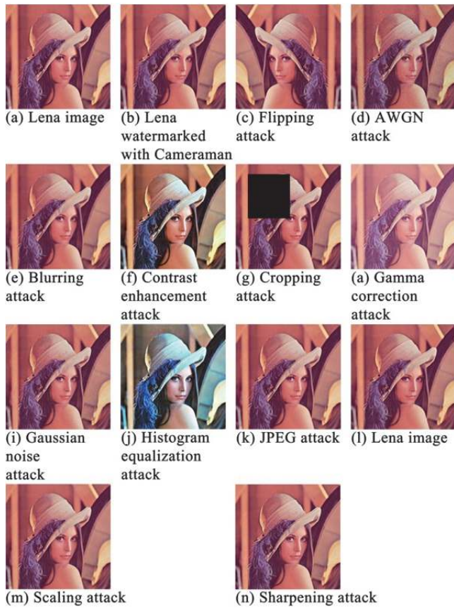
Fig. 4. (a) is the original image with size of 512 \times 512 , (b) is the original image watermarked with “Cameraman” image, (c-n) are watermarked images with different attacks.
