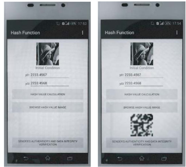
Fig. 12. Android application user interface : (a) image input for hash value calculation (b) displaying calculated hash value image in PNG format.
