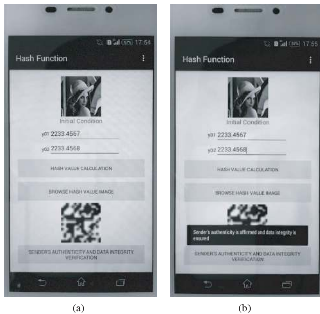
Fig. 13. Android application user interface : (a) image input for verifying sender's authenticity and data integrity (b) displaying results of sender's authenticity data integrity verifications.
