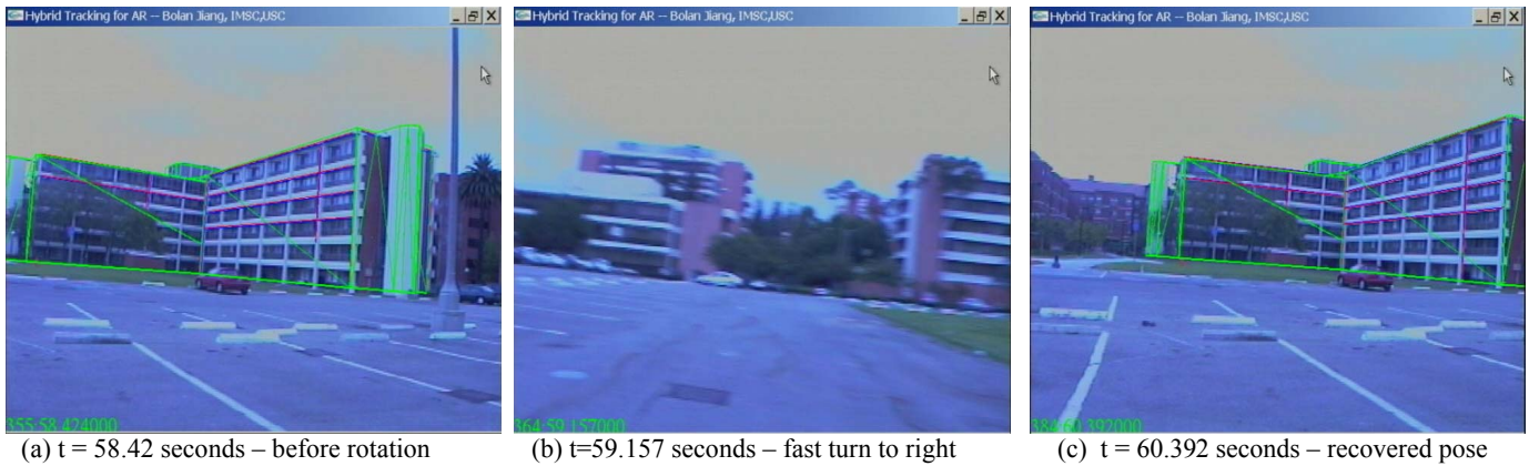
Figure 8 – Images from the second real-time experiment. The camera rotates away from the buildings. The green wire-frame is a 3D augmentation of the building. Red lines are the detected lines. Left bottom corners show the frame number: time stamp. The whole sequence has multiple rotations in different directions and lasts about 104 seconds. (a) Before rotating away. (b) After the modeled buildings are out of view. (c) Rotation back and automatic recovery of accurate pose.
