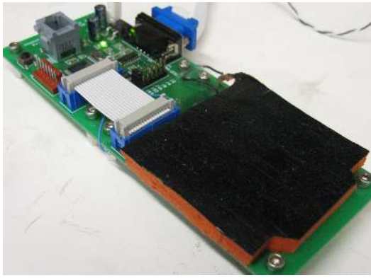
Fig. 8. The complete 4x4 sensor array with row-column addressing and sensor communication board attached
