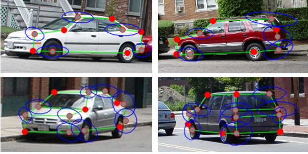
Figure 2. The partial shape Y_p (red dots) is used to hallucinate the remaining shape Y_h (gray dots). The marginal variance of the hallucinated points can be calculated and shown here in ellipses.
