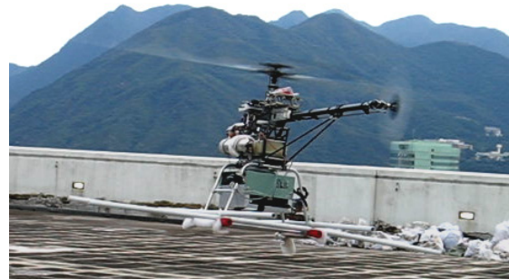
Fig. 1: The fully instrumented JR Voyager GSR260 for experiments. The IMU is mounted on wire-ropo isolators to avoid saturations.
