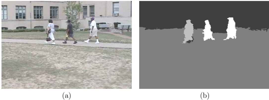
Figure 6.1: Layer segmentation of a sample frame in a short video sequence where three persons are walking on a road in front of a building. (a): One frame in the walking-people sequence. (b) Layer segmentation.
