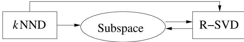
Figure 4.2: Three integrated components in our layer extraction algorithm. Subspace is the core component.
