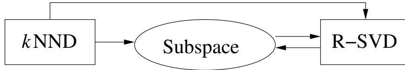
Figure 1.6: Three integrated components in semi-progressive layer extraction algorithm. Subspace is the centering component.
