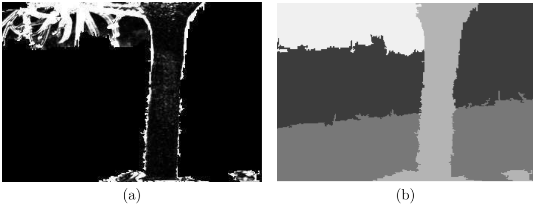
Figure 5.11: Progressive layer extraction. (a) Integrated residual image of the tree layer; (b) final layer segmentation.
