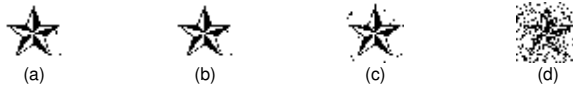
Fig. 8: The extracted watermarks from JPEG encoded versions of the SCHT watermarked Lena image (a) at 50% quality with NC \cong 1.00 , (b) at 40% quality with NC \cong 1.00 , (c) at 30% quality with NC=0.98 , and (d) at 21% quality with NC=0.80 .
