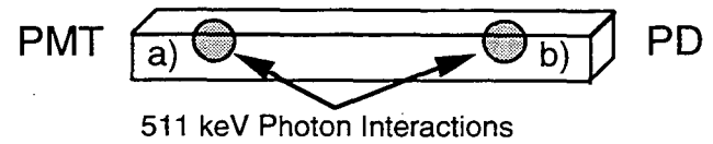
Figure 1: Depth of interaction measurement method. The scintillator crystal is coupled to a photomultiplier (PMT) and a photodiode (PD) and the other faces coated with a "lossy" reflector. Interactions near the PMT, as in a), result in a large PMT signal and a small PD signal. Interactions near the PD, as in b), result in a small PMT signal and a large PD signal.
