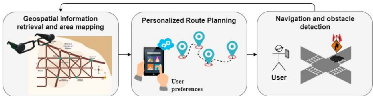
Fig. 2 Example of the use of route planning with a wearable assistive system
