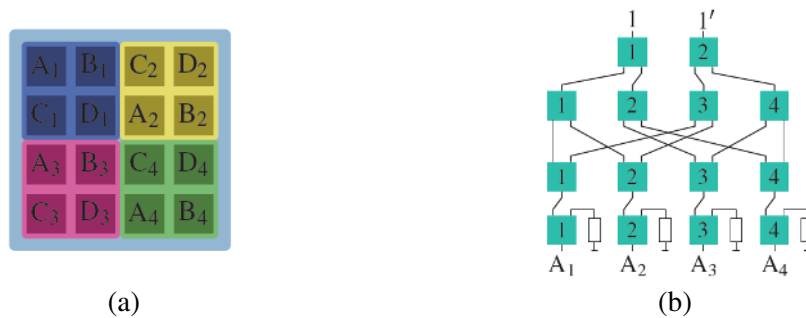
Figure 15. Concept of the switch matrix for the demonstration system. (a) Division on 2 \times 2 subarrays. (b) Schematic view of a switch module.
