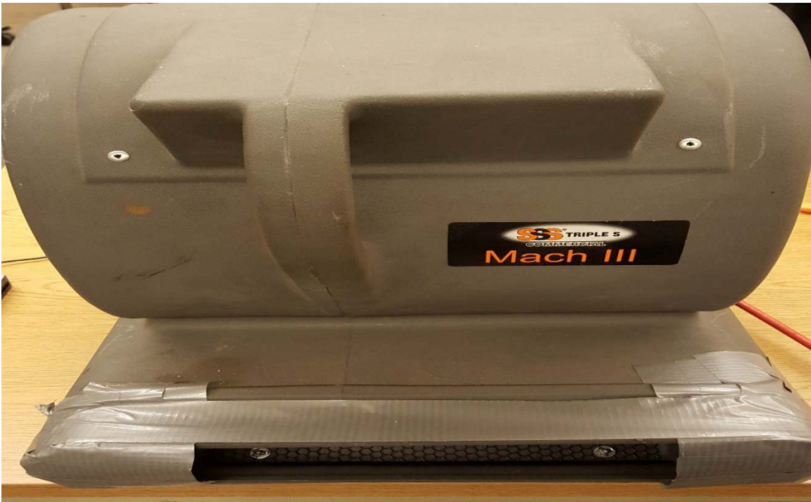
Figure 5.9: Blower Used for Wind Turbine.
