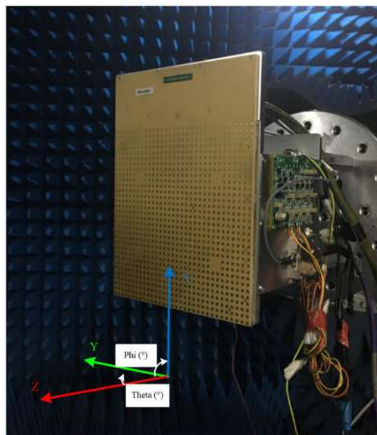
FIGURE 19. The 1024-element transmit phased array tested in anechoic chamber.
